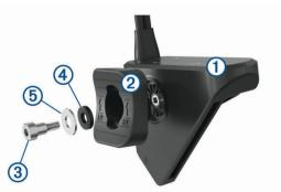
**2** Using the included hex wrench, attach the bracket to the transducer with the shoulder screw ③, rubber washer ④, and flat washer ⑤.
