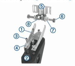
2 Attach the transducer mount bracket to the transom mount bracket ⑤ using the bolts ⑥, flat washers ⑦, and lock nuts ⑧.
