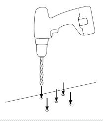
Use a 1½" to 2" (38mm to 50mm) hole saw for the center cable hole.
