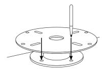
Using a 5/16" (8mm) drill bit, drill the four base bolt holes and center cable hole.
