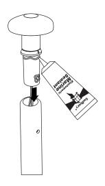
Secure the LTBU or LTBUSS with the two black push pins.
