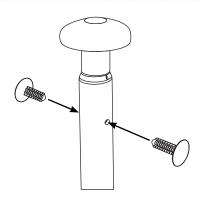
When securing make sure that LTBU or LTBUSS is facing forward. To check this line up the notch on the LTBU or LTBUSS with the hole on the back of the light bar as shown.
