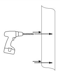
Using a 25mm hole saw, drill into the center of the mast to run our electronic cables.
