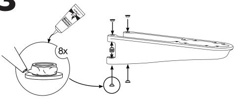
Once all shoulder washers are inserted attach the two mast mount feet.
