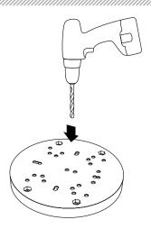
Secure the thermal camera to the adapter plate with the six M6x16 bolts and washers.
