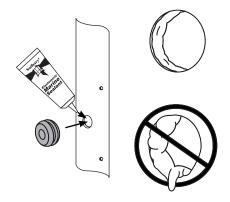
Apply Tef-Gel to the four holes you drilled for the mast mount feet. Again be sure not to apply too much.
