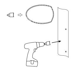
Apply marine adhesive sealant in the hole you just drilled. Be sure not to apply too much. Then insert the rubber grommet.
