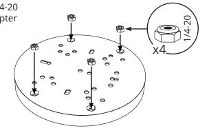
Place the drill template onto the adapter plate and mark the appropriate holes for drilling. Refer to the last page to find out which holes you need to drill.
