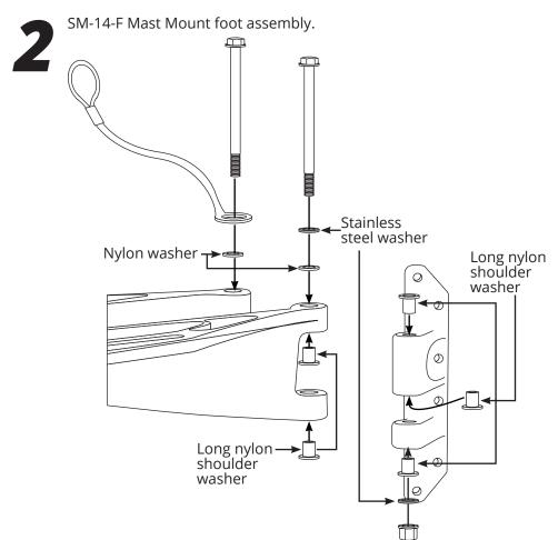
Apply marine adhesive sealant to the eight shoulder washers, then insert them into the mast mount as shown.
