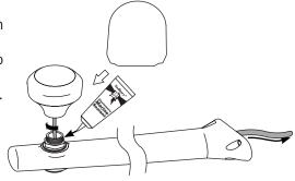
If you are using a closed dome radar use the provided plastic extion rods. Apply marine adhesive sealant to the threads of the adapter and screw on the GPS unit. Route the cables through the spreader.
