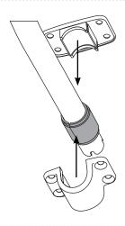
Place the white plastic spacer ontop of the adapter.
