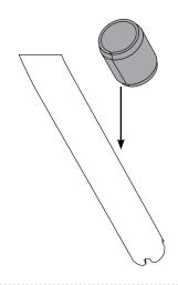
Place the white plastic adapter piece ontop of the rubber bushing.
