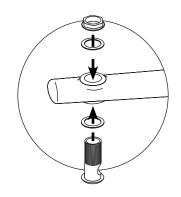
If you are using a satellite dome the plastic extension rod is not needed. Apply marine adhesive sealant to the threads of the adapter and screw on the GPS unit. Route the cables through the spreader.
